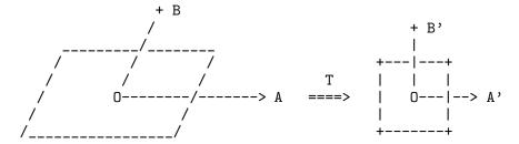
A = displacement vector along X-axis with length a
