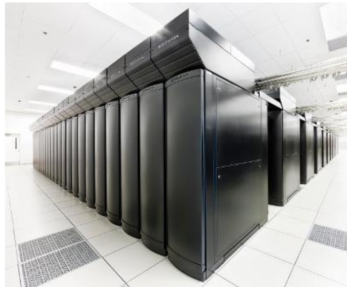
NCSA Blue Waters Hybrid Cray XE6 / XK7 22,640 XE6 dual-Opteron CPU nodes 4,224 XK7 nodes w/ Telsa K20X GPUs
