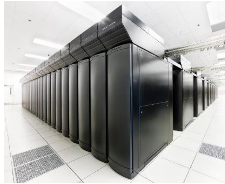
NCSA Blue Waters Hybrid Cray XE6 / XK7 Supercomputer 22,640 XE6 CPU nodes 4,224 XK7 nodes w/ GPUs
